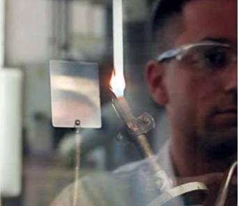
Flammability test (UL94) in the LuV laboratory: a sample of material without flame retardation (left) compared with halogen-free flame retardation (right).
